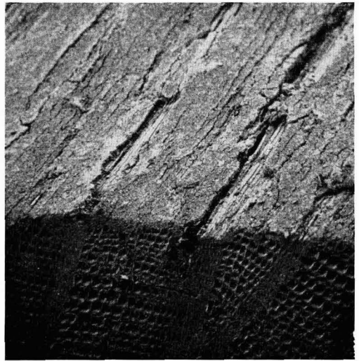
Figs. 4a (left) and 4b. Stereoscan photographs of sections through paint film and wood, showing association of cracking with junction of early and late wood.
