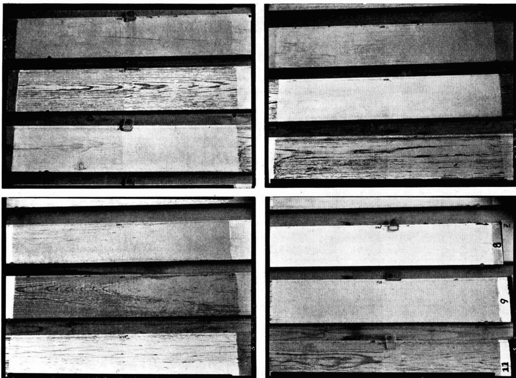
Figs. 2a (top left), 2b (top right), 2c (bottom left) and 2d. Section of primers, set 1 (one eighth actual size). The sections are contiguous parts of three complete boards
