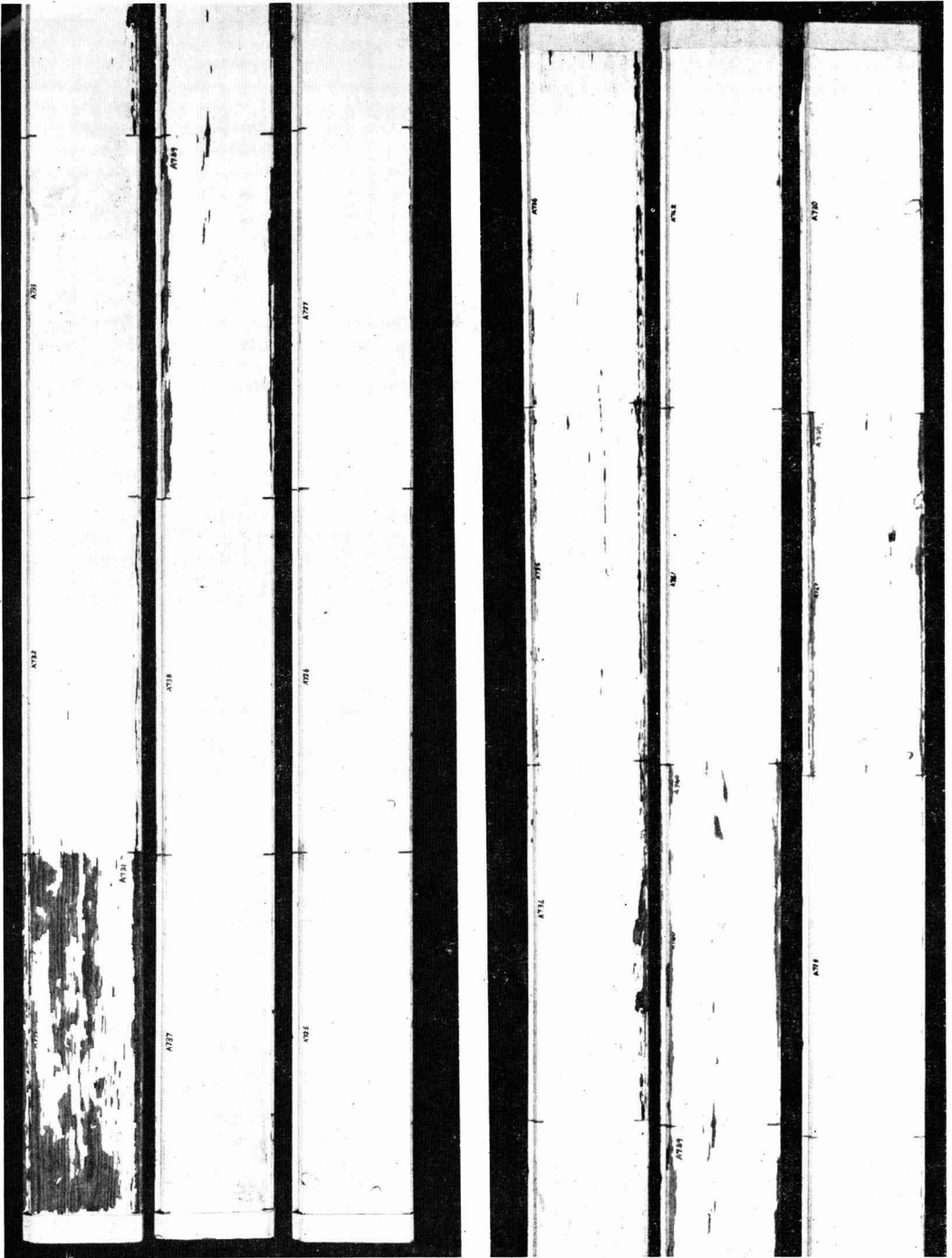
Figs. 3c (left) and 3d. Primers plus gloss coat after one year's exposure, corresponding to those in Fig. 2 (plus others). (N.B. Although the panels are shown vertical here, they were kept in the horizontal position during tests and photographing.)
