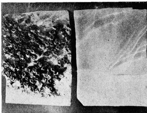
Fig. 2. Marine fouling by barnacles (Courtesy: Schering AG, Bergkamen, West Germany)
