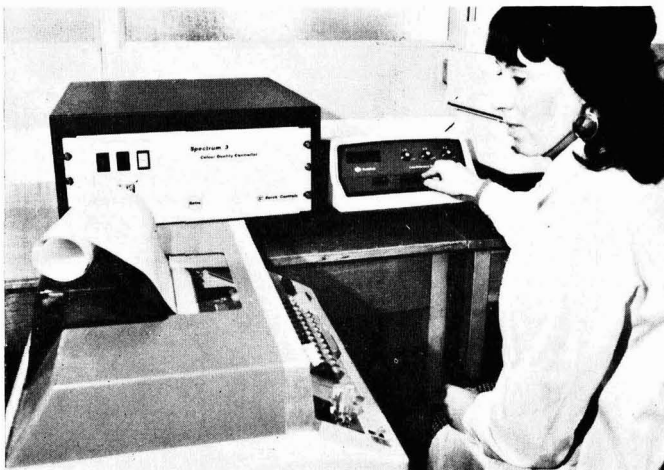
The system "Spectrum 3", a joint development between Serck Controls and Hatra, which facilitates colour quality control and repetitive colour production. Differences between a standard colour and colour samples can be readily measured and pass/fail decisions within customer's prescribed limits printed out in permanent record form
