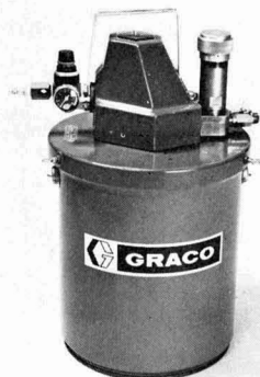
A patented airspray gun supply unit from Graco Ltd; the unit can be flush cleaned in approximately two minutes and is about one-quarter the weight of a conventional 20-litre pressure pot
