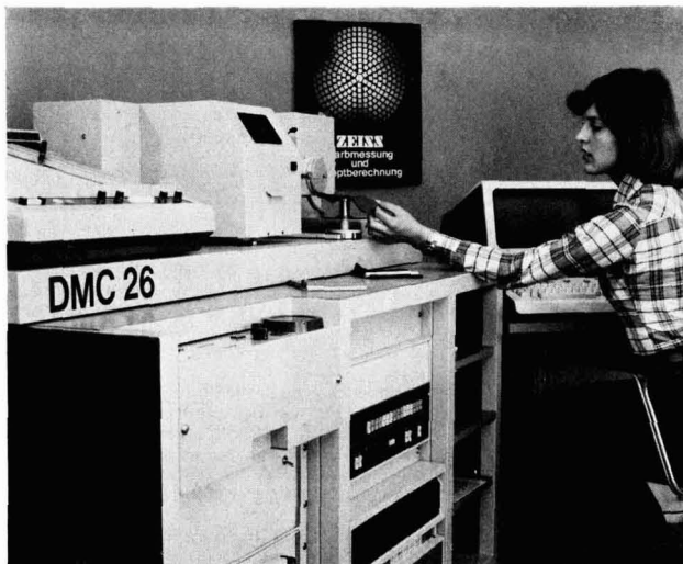
The DMC 26 colorimeter now available from Carl Zeiss. The company emphasises speed, high accuracy and reproducibility as features of the new instrument, which is claimed to be a "master instrument" for reflectance measurement and colour matching. Computer and digital plotter are from Hewlett Packard.
