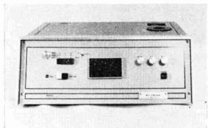
The "Du-Color" colorimeter for measurement of colour difference, opacity and brightness, shade differences, CIE X, Y and Z values, and absolute reflectance and transmittance
