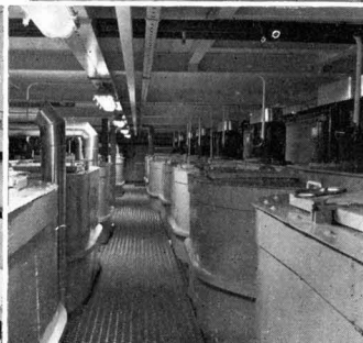
From the control room (left), the operator can supervise the simultaneous production of up to three bases and look through a window to (top) where the correct quantities of resin, solvent, etc are automatically metered into the mixing and dispersion vessels. The bottom right-hand photograph shows the tanks for storing the final bases
