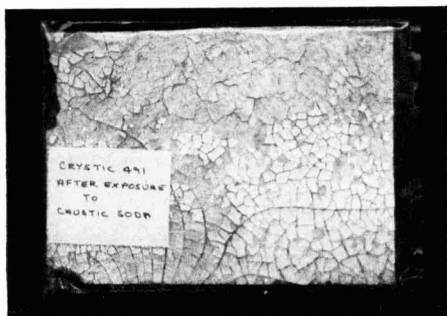
Fig. 3. Crystic 491 laminate after exposure to sodium hydroxide solution
