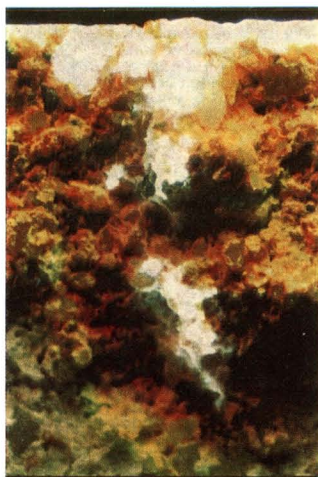
Fig. 9. Copolymer containing optical brightener in lime-sandstone (using a 20% emulsion)
