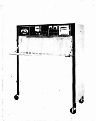
The "UVCON" unit for screening materials sensitive to ultraviolet light and condensation, which has been introduced by Atlas Electric Devices Co. (UK agent Wentworth Instruments Ltd)
