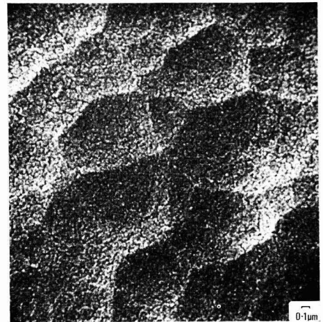
Fig. 7. Etched aluminium with developed porous surface (3L72)
