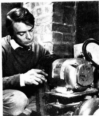
Electric motor with Thremindex Indicators fixed to the casing to give an early warning of impending troubles
