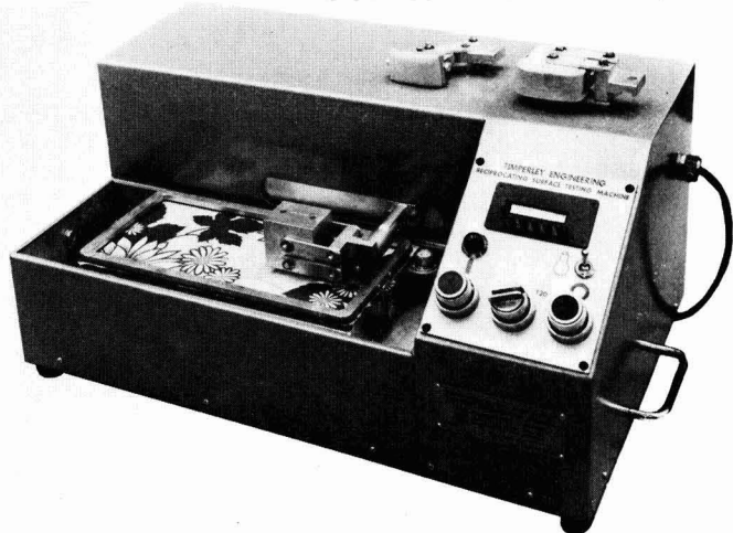
The new reciprocating surface tester from Timperley Engineering, which can be used to test the durability of coatings
