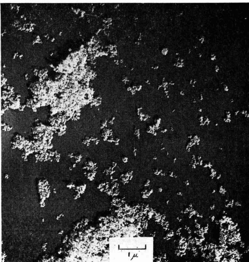
Fig. 1. Electron micrograph ( \times 20,000 ) Carbon black, poor dispersion
