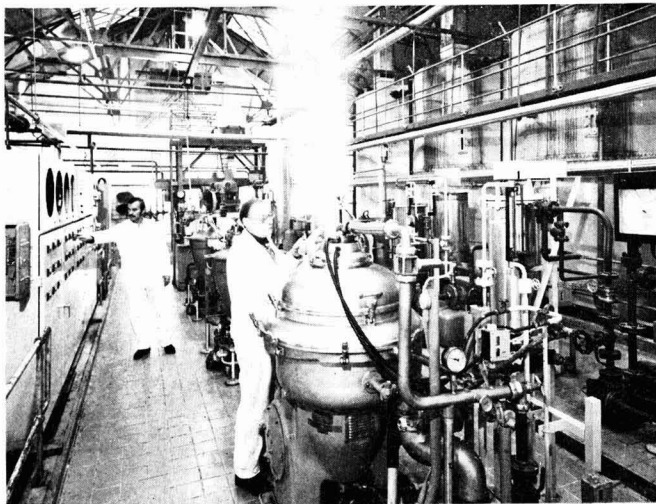
A view of the centrifuges and control panel at the new BOCM Silcock technical oil refinery
