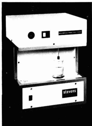
The new Boucher Electronic Jelly Tester, which measures gel strength
