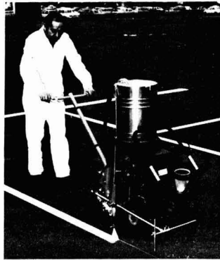
The line marking unit designed for use with a Wagner airless paint sprayer
