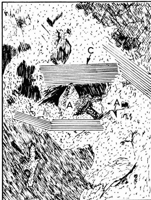
Fig. 1. Drawing from a microphotograph of the narrow molecular weight fraction of the alkyd that is discussed in the text. Crystalline regions are marked C. Amorphous regions are marked A.
