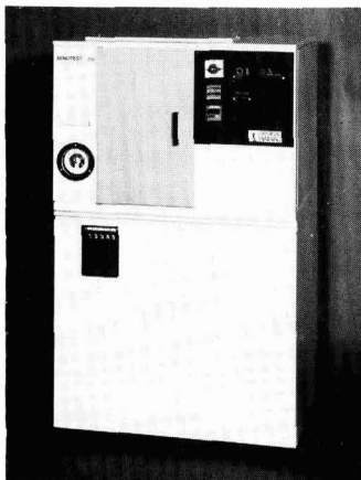
The Xenotest 250 light fastness testing and weathering machine
