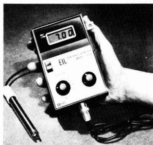
The new model 3050 hand-held digital pH meter from Electronic Instruments Ltd
