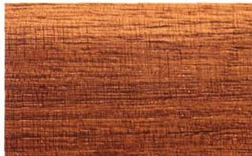
Nitrocellulose curtain-coating lacquer with 0.5% PERENOL E1
