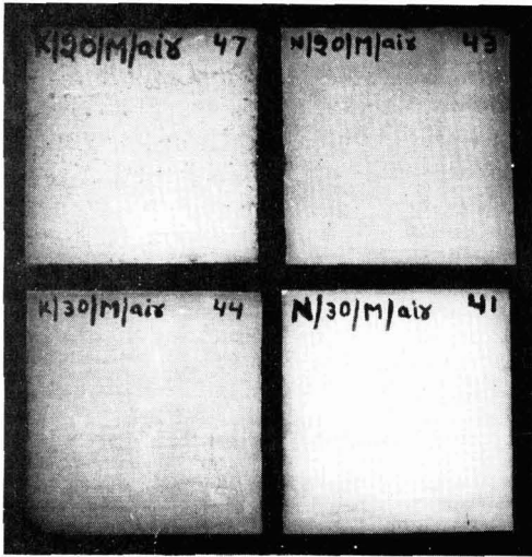
Figure 1. The performance of sodium and potassium silicate based paints and the effect of variation of the pigment content. All paints self-cured.
