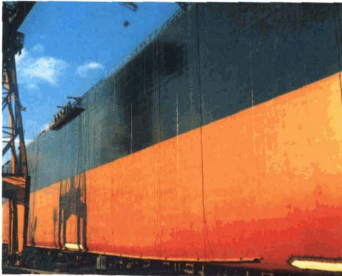
Figure 8. Side of a bulk carrier shortly before launching. The cradle used for painting is suspended from the deck (Photograph: Berger Paints)
