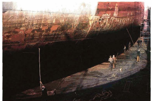
Figure 10. Scraping the side of a ship in drydock (Photograph: Berger Paints)
