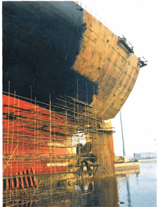
Figure 9. Stern of a bulk carrier shortly before launching. Cradles are used for painting at deck level, but staging is required for overhanging areas (Photograph: Berger Paints)
