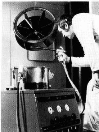
The Mindon tribo-charged airstatic powder spray gun
