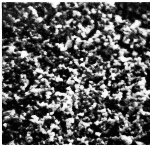
Figure 1. Long oil alkyd paint (Paint C): 2 years natural weathering - 25° view
