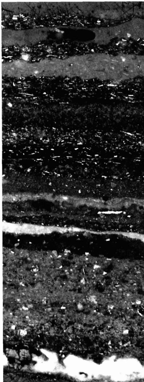
Figure 4. Cross-sectional examination of paint flake from Royal Albert Bridge, Saltash, Cornwall
