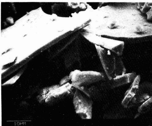
Figure 1. Comparison of the crystal structures of mica (top) and micaceous iron oxide (bottom)
