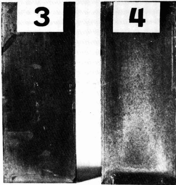
Figure 5. Weatherometer test (200 hrs); Panel No. 3 Process - 3, Panel No. 4 Process - 4
