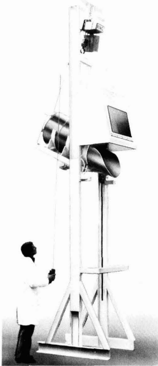
The WS Liftips drum handling equipment for controlled discharge
