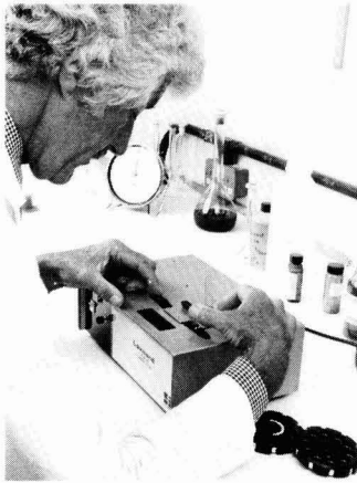
Improvements to the Lovibond Three-Field Comparator include: slot-in discs of Lovibond glass colour standards and a new prismatic viewer
