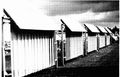
Figure 9. Test stand modified to retain coil-coated siding with eave overhang
