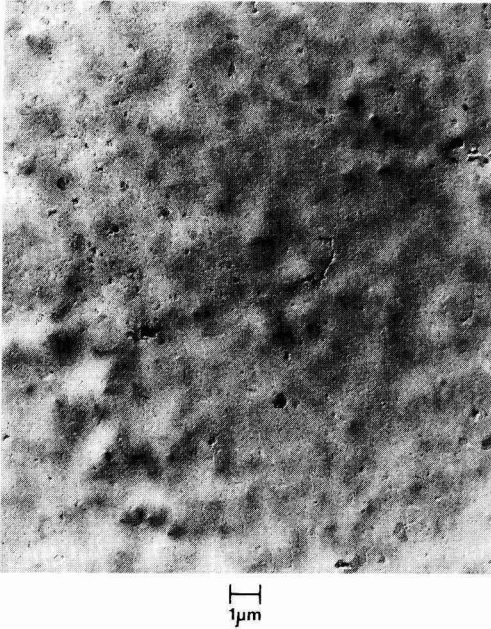
Figure 12. An electron micrograph of the surface (replica) of an acrylic water-based coating containing 0.05% catalyst
