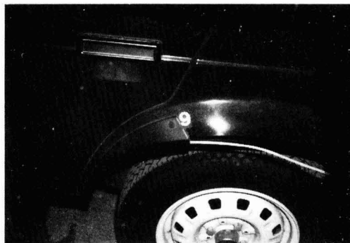
Figure 1. The outward flared rear wheel arch is protected by a plastic guard to reduce claims under the paint warranty. The plastic tube highlights the crevice produced between the plastic and the car body
