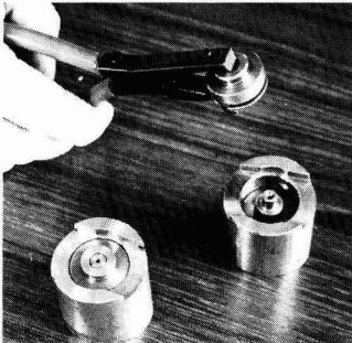
Clayton-Heyes' high pressure threadless spray nozzle
