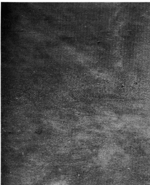
(b) 5:1 ( 2.5 \times 10^{-4} \text{ mol dm}^{-3} : 5 \times 10^{-5} \text{ mol dm}^{-3} ), 1000 \times Figure 6. SEM of paint films containing various mole ratios of SDS/SHMP
