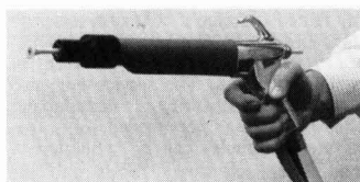
Mindon's new electrostatic spray gun showing double moulded barrel, delicate electrodes contained in a separate nozzle which will push into the main barrel, and liquid filled high voltage cable
