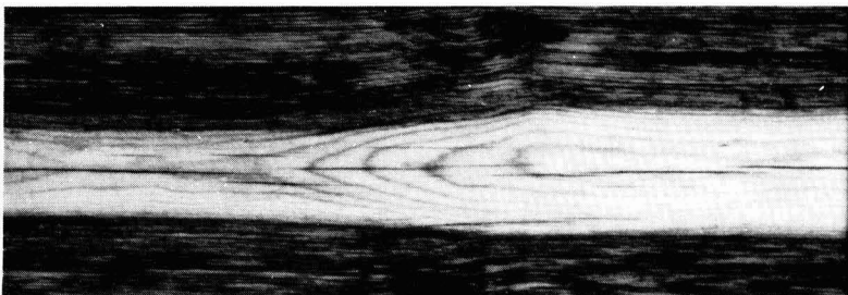
Figure 10. Blue stained pine sapwood, primed with an impregnating agent
