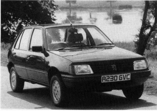
Figure 3. The newly introduced Peugeot 205 has a comprehensive anticorrosion specification based upon the use of zinc pre-coated steels, which account for over 40 per cent of the body weight
