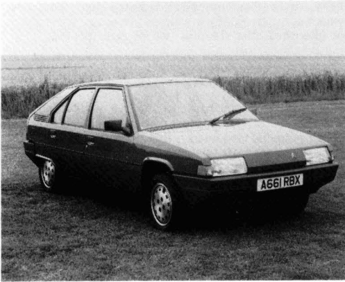
Figures 1. (Left) and 2. (Right) The Citroen BX embodies bonnet, tailgate and other panels in reinforced plastics materials
