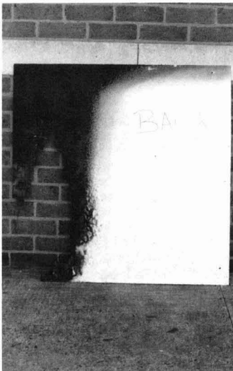
1. Panel painted with two coats of solvent-based intumescent paint and high build decorative finish
