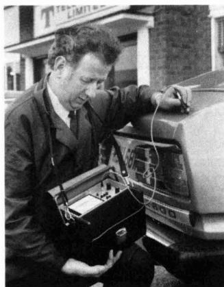
The Leptoskop 2012 from Teledictor being used to check paint layer thickness
