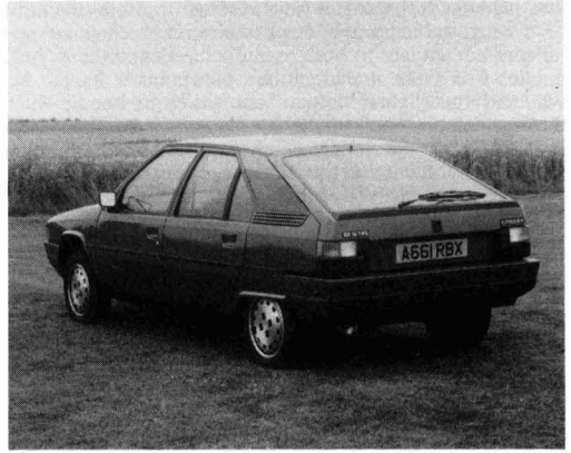
Figures 1. (Left) and 2. (Right) The Citroen BX embodies bonnet, tailgate and other panels in reinforced plastics materials
