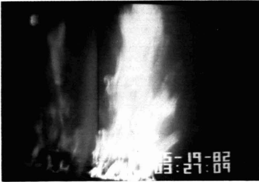
1. Surface flame flashing
