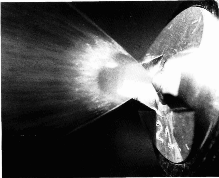
Figure 1. High paint-pressure atomisation
