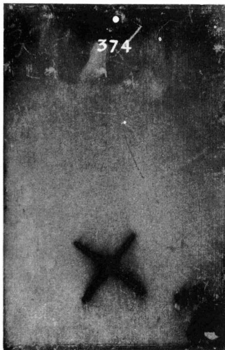
One coat red lead primer to BR Specification 35 Item 8, one coat micaceous iron oxide undercoat to BR Specification 35 Item 61, one coat micaceous iron oxide finish to BR Specification 35 Item 62. Panel exposed 1 January 1964; only primer was brush applied other coats were sprayed
