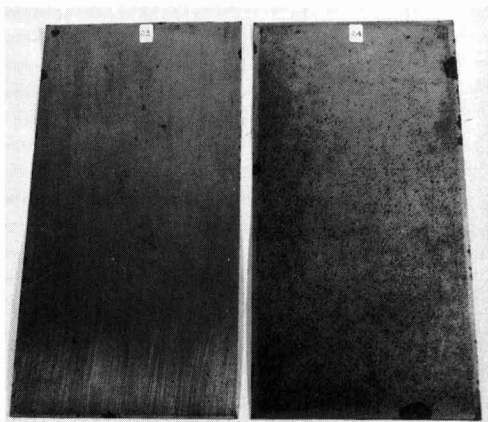
Figure 22. Surface condition of steel panels after 80 days of weathering tests. Both test panels (23 and 24) were coated with epoxy resin-based paint pigmented with either MIOX (test panel No. 23) or SA MIO (test panel No. 24)
