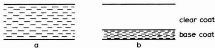
Figure 1. Paint film compositions of conventional metallic (a) and base coat/clear coat (b) systems showing the different aluminium flake distribution
