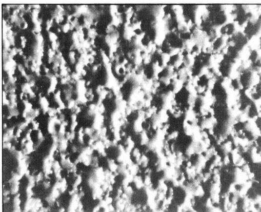
Figure 5. Higher power (100X) photograph of unbaked high build primer over zinc phosphated cold rolled steel. Typical rough and bumpy but fairly regular surface.
