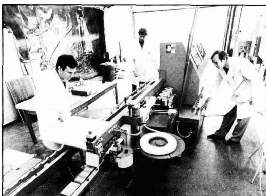
Assessment of the operation of an edge banding machine using PVAC adhesive
