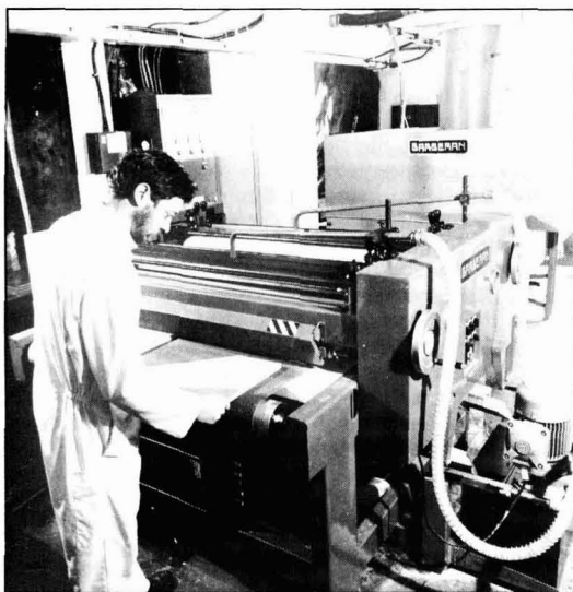
Roller coater and UV oven being assessed in the FIRA pilot plant area
