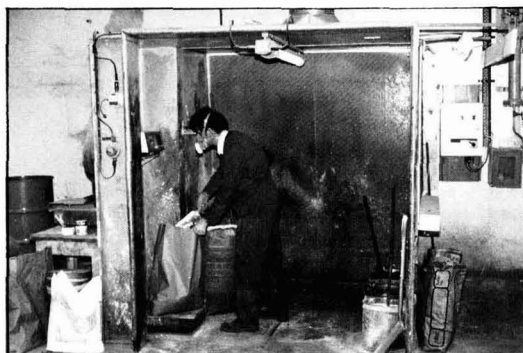
Figure 3. Operator weighing out small quantities working in a laminar flow booth and wearing a dust mask.
