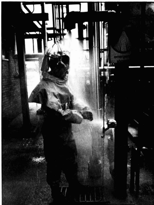
Figure 2. Shows a fully protected operator at the decontamination shower after supervising the unloading of a TDI bulk tanker.
