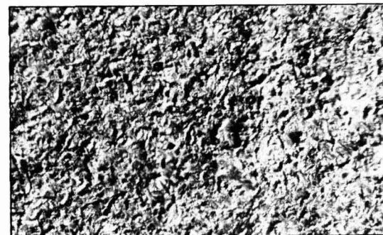
Figure 3. Galvanized surface blasted with grade G12 chilled iron grit. Magnification x30.
