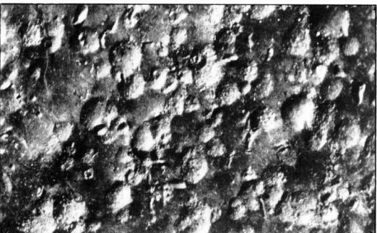
Figure 8. Galvanized surface blasted with grade S240 chilled iron shot. Magnification x30.
