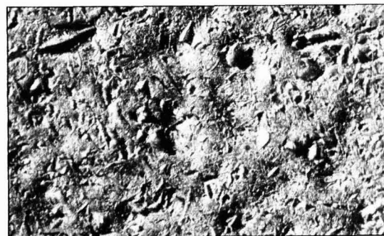
Figure 2. Galvanized surface blasted with copper slag. Magnification x30.
