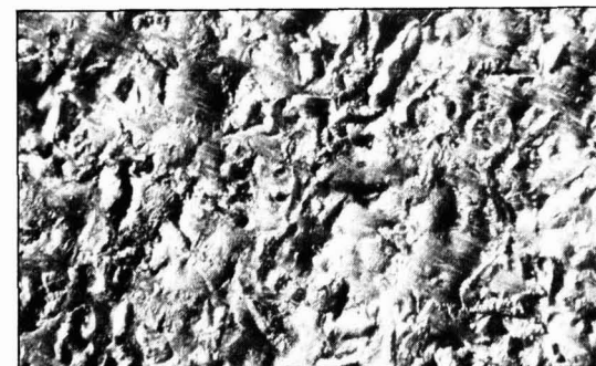
Figure 4. Galvanized surface blasted with grade G24 chilled iron grit. Magnification x30.
