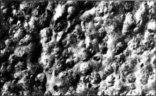
Figure 7. Galvanized surface blasted with grade S120 chilled iron shot. Magnification x30.
