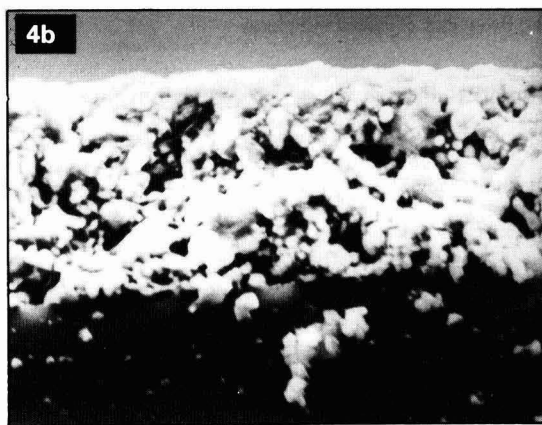
Figure 4. SEM micrographs of cross-section of a dry film of epoxy polyamide zinc-rich paint: (a) of distilled zinc dust at a 92.9% loading, (b) of atomized zinc dust at a 89.5% zinc loading (magn. \times 850 ).
