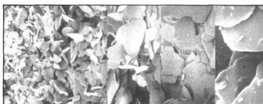
M F N S L TiO 2 - MICA PLATELETS OF DIFFERENT PARTICLE SIZE DISTRIBUTION M: 1 - 15 MICRON (90%) F: 5 - 20 MICRON (90%) N: 10 - 50 MICRON (90%) S: 10 - 130 MICRON (90%) L: 40 - 200 MICRON (90%) THICKNESS: 0.1 - 0.5 MICRON
