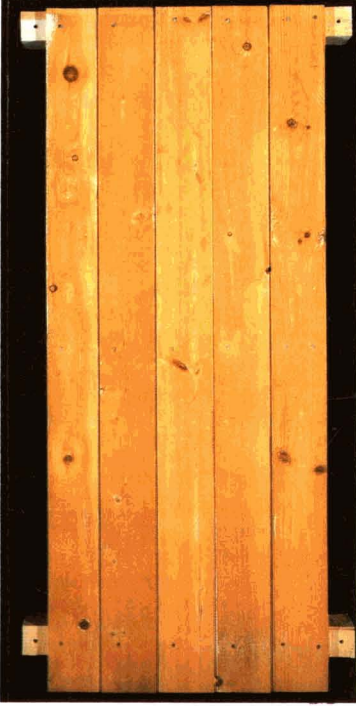
Figure 3 Appearance of assemblies cleaned by sand-blasting
