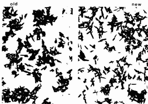
Figure 7. Electron microscope photos of the new highly stabilized Dark Chrome Yellow (right) vs the corresponding previous product (left).
