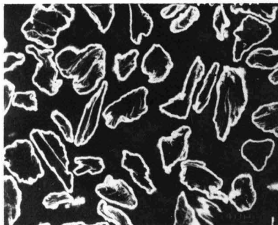
Figure 5 Structure of typical nickel-coated graphite particles.
