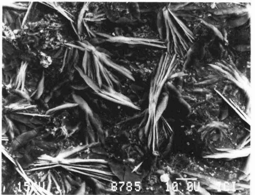
Scanning electron micrograph of "Generation II" zinc phosphate (x2000).
