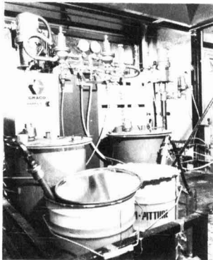
The Graco Hydra Cat mixes the two-pack coatings.
