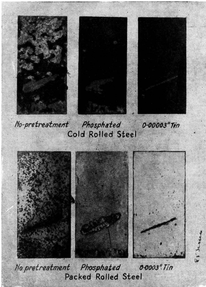
Fig. 3.—Cold rolled and pack rolled steel plates painted after various pretreatments and exposed for 1,500 hours to accelerated weathering tests. The lower set of photographs were exposed for 1,500 hours to accelerated weathering tests. The lower set of photographs were taken after stripping the point and removing the phosphated coating to exhibit the extent of rusting.
