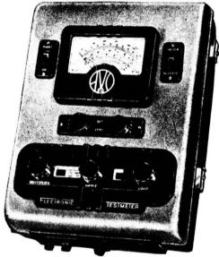
D.C. Volts: 2.5~mV. to 250~V. (Input Resistance III-0 megohms.) 25~mV. to 10,000~V. (Input Resistance III0-0 megohms)
