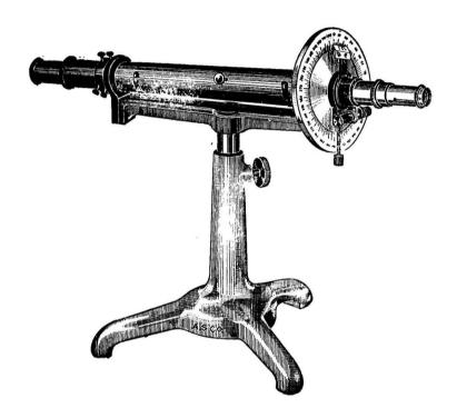
Fitted with Lippich device which makes the instrument sufficiently accurate and at the same time simple. Can be used with sodium burner or an electric lamp with suitable filter interposed into position between the source of light and the polimeter.
