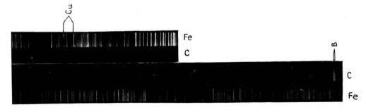
Fig. 4 — Cathode layer spectrum of carbon rod purified by resistance heating.
